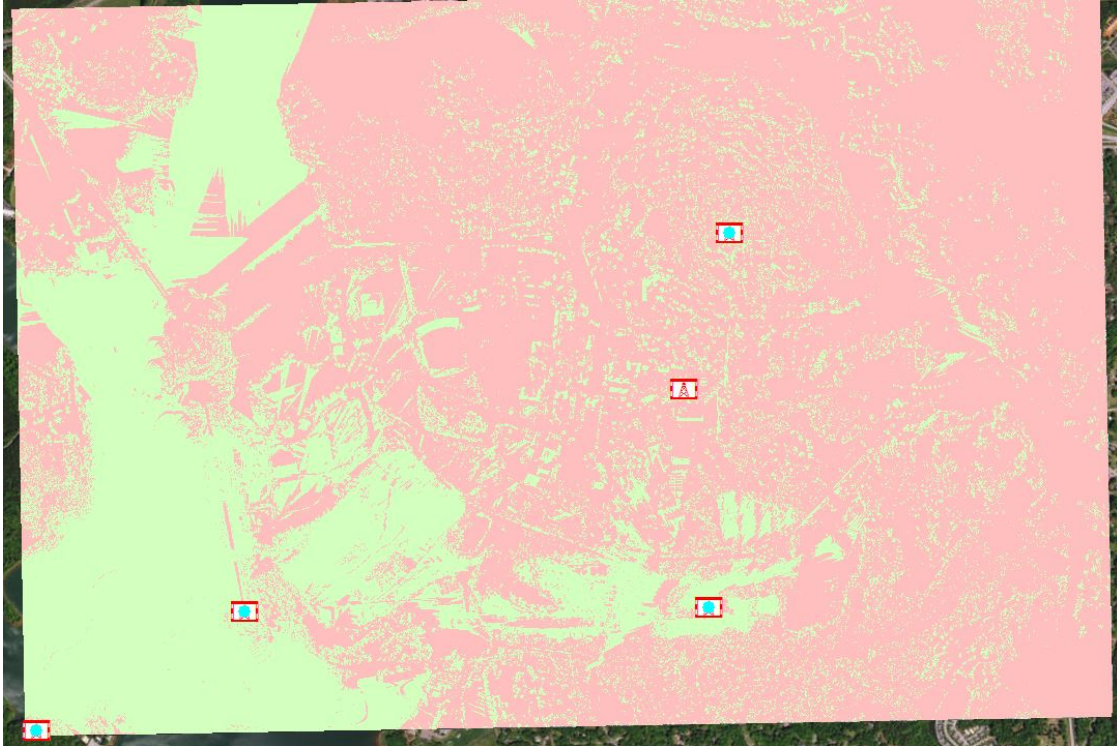
Figure 27. The original viewshed. Green areas are visible from the current cell towers and red areas are not visible.
