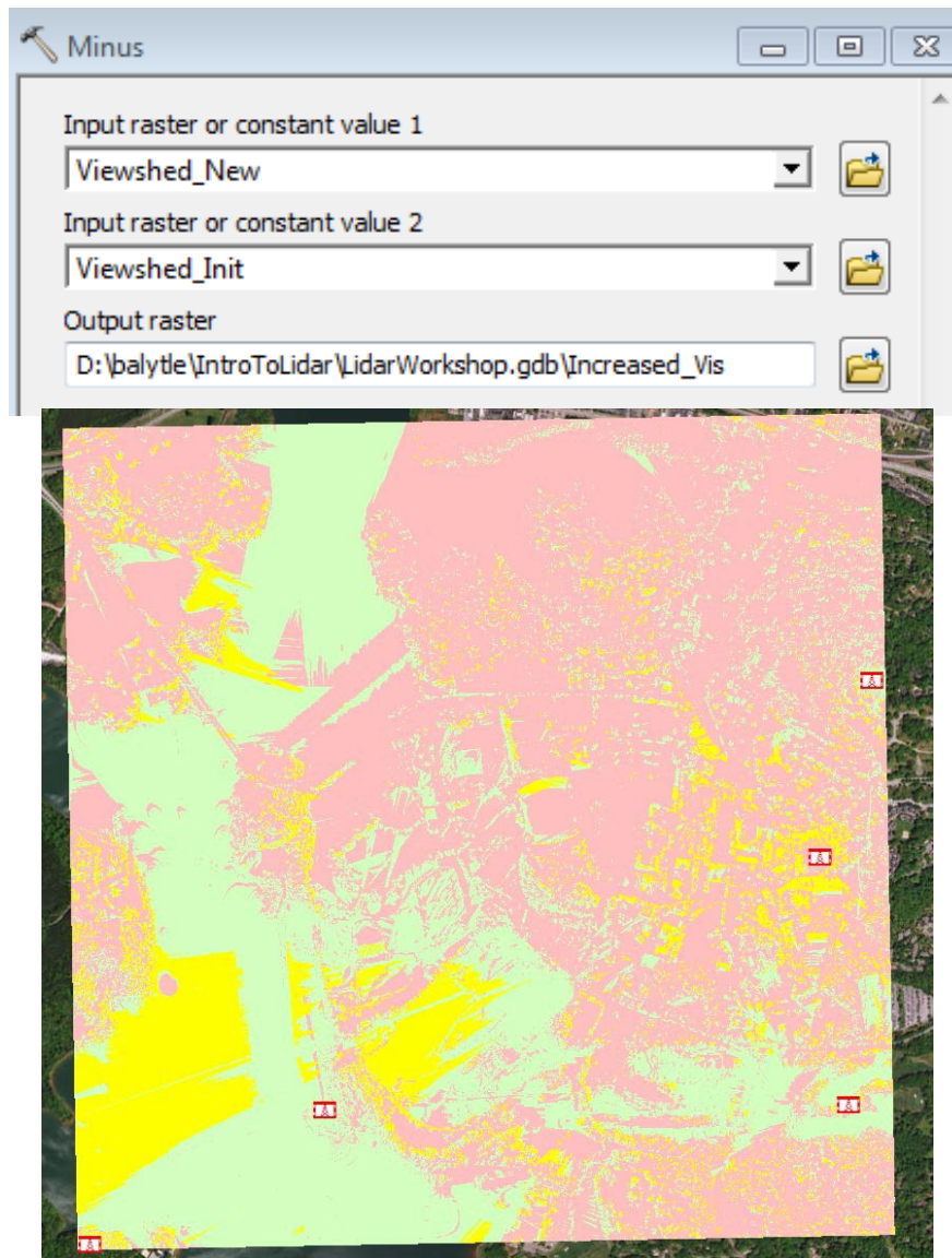
Figure 29. The Minus tool settings (above) and the areas of increased cell visibility from the new tower (below).
